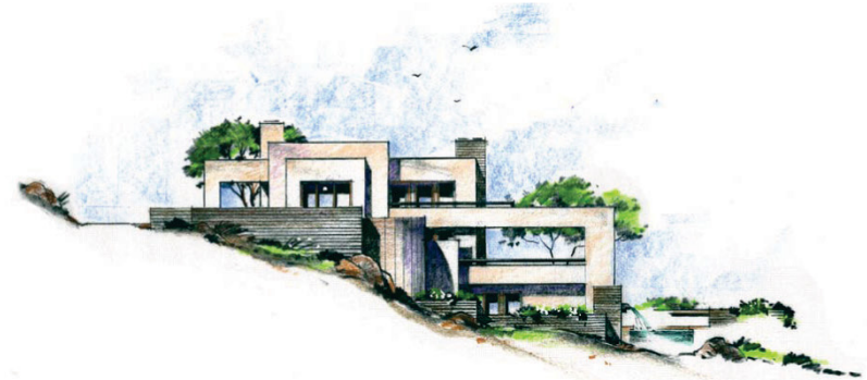
Steep downhill grade adaptive design reflecting a 20% to 30% grade and multiple levels.
