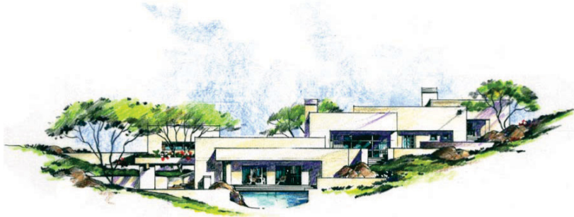
Swale or valley condition illustrating grade adaptive design utilizing the low portion of this building envelope.
